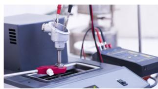
Range of equipment suitable for verification and validation measurement procedures to ensure product quality and constant optimization of probes and transmitters.
