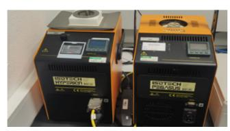
Dry and oil bath furnaces are high precision and stability equipment used in validations and internal characterizations.
